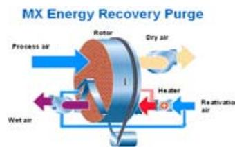
The unique patented Munters Energy Recovery Purge system acts as an energy recovery system, collecting waste heat from the hottest section of the desiccant wheel and using it to help with the regeneration process. This reduces the energy required for reactivation while lowering the discharge temperature of the process air, decreasing energy costs for post cooling.
